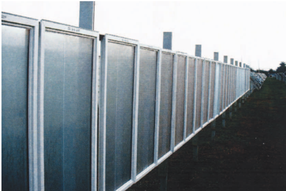
Outdoor exposure of Preserve Masking test units (Arizona – Top Florida – bottom)
